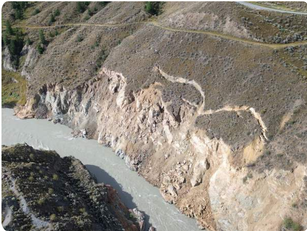
Photo 2 (left): Visible tension crack at Nagwentled (Farwell Canyon) on Sept 13, 2025. A BGC Engineering report identified a high risk of hillslope failure and rockfall in the short-term due to erosion. This is already a challenging area for salmon to pass, and a central fishing site for the T̄silhqot̄'in Nation. Rockfall poses a high risk of impediments to salmon passage. (Photo courtesy of BGC Engineering).
