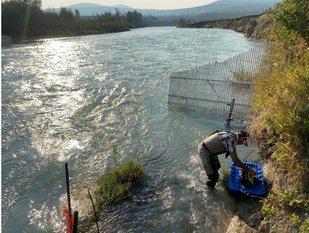
Figure 2. TNG fisheries technician Gerald Williams performing daily maintenance at river-right bank Hanceville sonar station. Captured on Sep 01, 2025.
