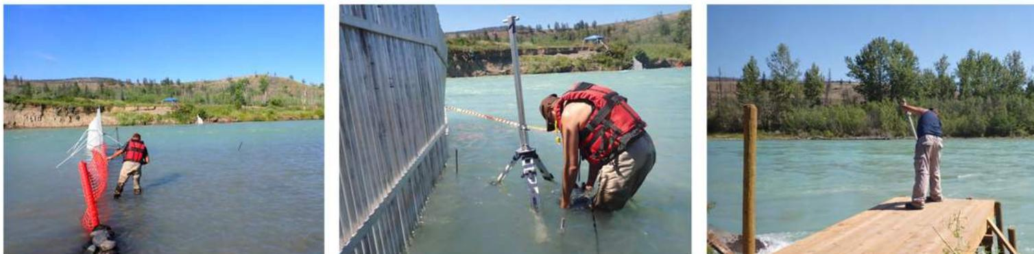
Top left & middle: TNG Sr. Fisheries Technician Gerald William performing standard maintenance at the Hanceville SONAR, including cleaning the diversion fence (left) and the SONAR lens (middle).
