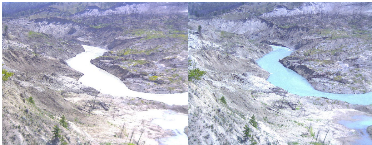
Figure 7 Recent bank movement at the landslide area. Photo on the left captured June 10, 2025 and photo on the right captured July 04, 2025.
