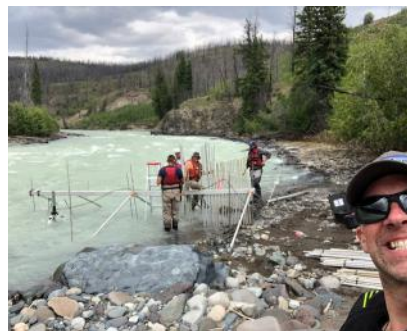
Photo 2: Fisheries Biologist Pete Nicklin and the TNG and DFO crew installing the Taseko SONAR system to count Ts̓eman (sockeye) and Ja̓s (Chinook) migrating through the Taseko River.
