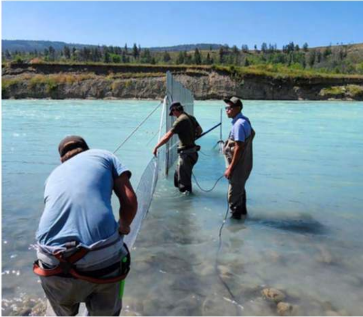
Above: Leonard English and Winston Bambrick of TNG Fisheries with Ecofish and DFO technicians installed a new SONAR just above the slide site (at Hanceville) Aug 8 to detect when fish start passing through the slide. The SONAR is operating continuously and staff are reviewing and reporting results in near-real-time.
